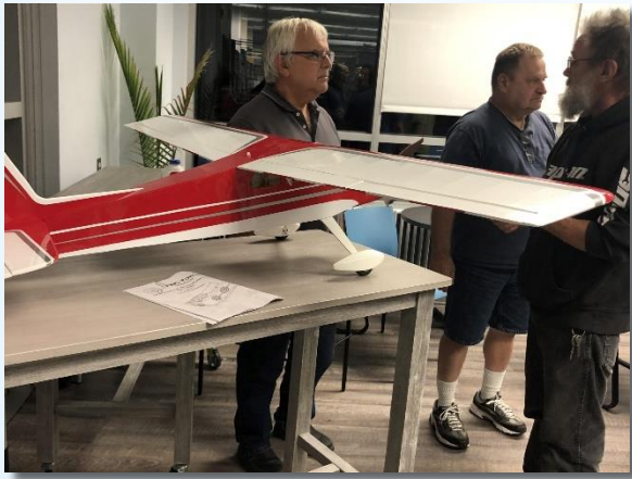
Dan Vensel's Hangar 9 10cc ARF with Power 46 motor, six MG servos, 96" wing, 12x8 prop, two 4 cell lipos in parallel totaling 8,000 mah.
