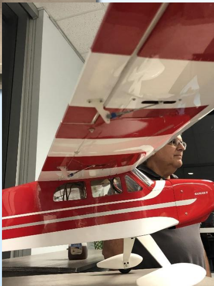
Dan Vensel's Hangar 9 10cc ARF with Power 46 motor, six MG servos, 96" wing, 12x8 prop, two 4 cell lipos in parallel totaling 8,000 mah.
